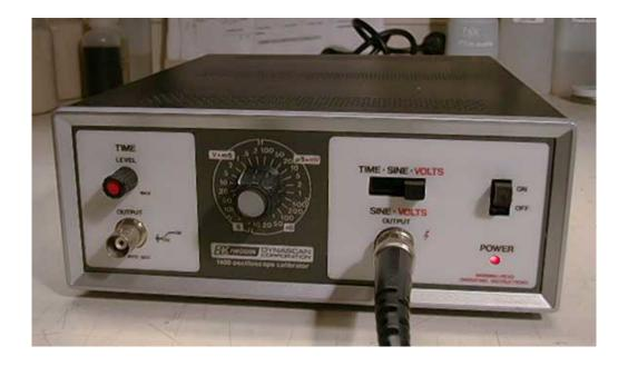
**Model 1400 Oscilloscope Calibrator**
