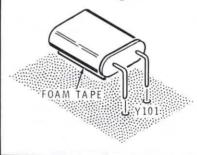
) Y102: Similarly, use the remaining 3/8" piece of double-stick foam tape and mount the 20 MHz crystal (#404-651) at Y102. Solder the leads to the foil and cut off the excess lead lengths.
